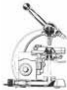
Illumination device with separate control of the luminous field and condenser aperture: August Köhler 科勒照明的提出
